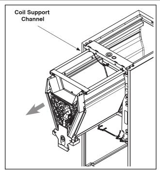
**STEP 5** - For extremely tight spaces where the cabinet needs to be rotated through a small opening, remove the top panel and all cross members. Use a manual driver to avoid stripping screw holes.
