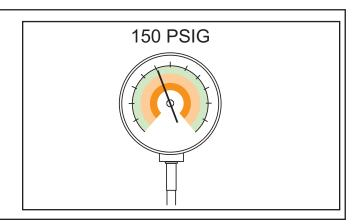
**STEP 10** - Check for leaks by using a soapy solution or bubbles at each brazed location.
