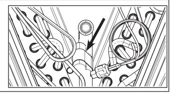
**Important:** Do not open the service valves until the refrigerant lines and indoor coil leak check and evacuation are complete.
