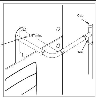
**STEP 5** - Insulate the primary drain line to prevent sweating where dew point temperatures may be met. (Optional depending on climate and application needs.)
