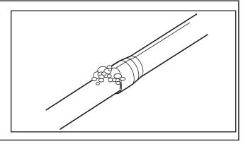
**STEP 11** - Place the TXV sensing bulb back into the clip on the Vapor Line. Insulation over the TXV bulb is not required.
