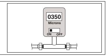
**STEP 13** - Observe the micron gauge. Evacuation is complete if the micron gauge does not rise above 500 microns in one (1) minute.
