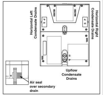
**Note:** A small amount of sealant must be applied around the drain line(s) passing through the panel to prevent air leakage and possible water drips.
