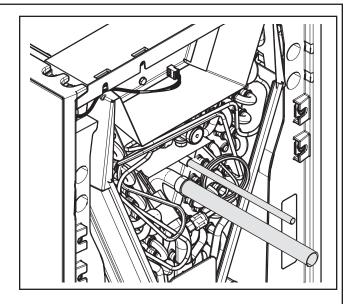
**STEP 9** - Pressurize the refrigerant lines and evaporator coil to 150 PSIG using dry nitrogen.
