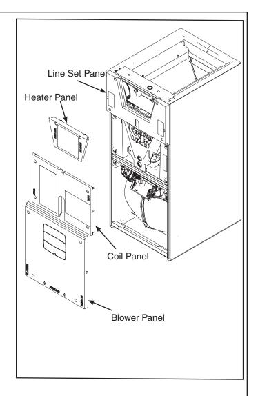
**IMPORTANT:** Removal of the Line Set Panel is required for all refrigerant line brazing and some condensate line assembly depending on your orientation.
