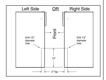
**Note:** Strain relief must be provided on the inside of the air handler cabinet for the low voltage wiring. Field supplied thermostat wires may be wire tied as a bundle to the existing strain relieved low voltage pigtail leads in the air handler unit.
