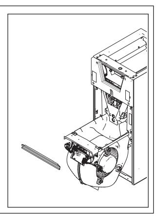
**STEP 3** - Slide Blower assembly out of unit using built-in blower support channels and set aside.
