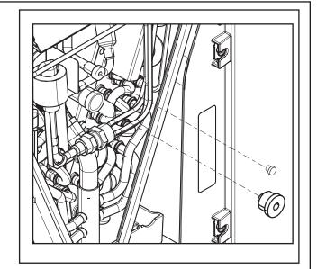
**STEP 7** - Connect, but do not braze, field line set to indoor coil.
