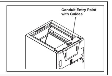
**STEP 3** - Route conduit (if used) to the entry point and connect.
