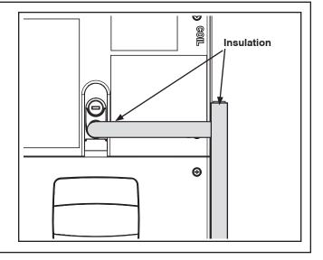
**STEP 6** - Support the condensate piping outside the unit per local codes for proper drainage and to prevent sagging.
