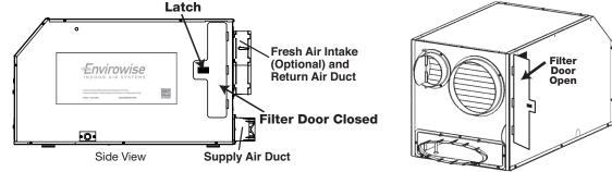
**Step 2:** Remove the filter by gently pulling it straight out of the unit. Insert new filter by gently pushing it straight into the unit. Make sure the AIR FLOW arrow on the filter is pointing into the unit.
