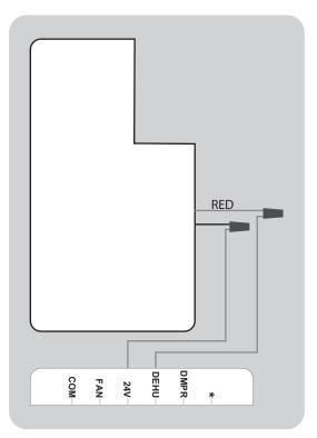
A 24V control must be used with the Envirowise XT155H.
