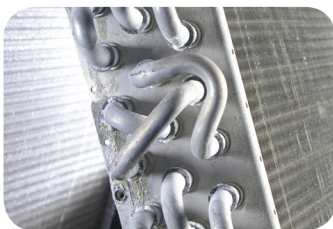
Aluminum tube and tube sheet after 500 hours in a controlled corrosive environment.
