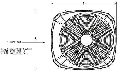
TOP DISCHARGE AREA SHOULD BE UNRESTRICTED FOR AT LEAST 1524 (5 FEET) ABOVE UNIT. UNIT SHOULD BE PLACED SO ROOF RUN-OFF WATER DOES NOT POUR DIRECTLY ON UNIT, AND SHOULD BE AT LEAST 305 (12") FROM WALL AND ALL SURROUNDING SRUBBERTY ON TWO SIDES. OTHER TWO SIDES UNRESTRICTED.
