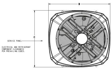
TOP DISCHARGE AREA SHOULD BE UNRESTRICTED FOR AT LEAST 1524 (5 FEET) ABOVE UNIT. UNIT SHOULD BE PLACED SO ROOF RUN-OFF WATER DOES NOT POUR DIRECTLY ON UNIT, AND SHOULD BE AT LEAST 305 (12") FROM WALL AND ALL SURROUNDING SHRUBBERY ON TWO SIDES. OTHER TWO SIDES UNRESTRICTED.
